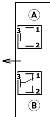
*Top View. The arrow indicates the glass side where the sensor is mounted on TK3 body. The 90° female flying part exit on the other side.*
